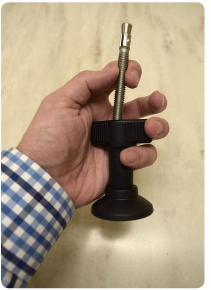
7. Insert the 3/8" thread bolt from the side arm package into the tightening handle from the Manfrotto tripod.
