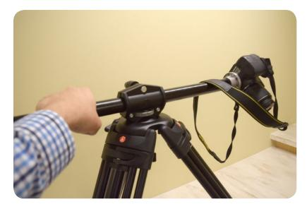
**13.** Turn the pole to the desired angle and then tighten the lever.
