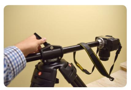
**12.** Turn the lever on the sidearm to loosen the pole
