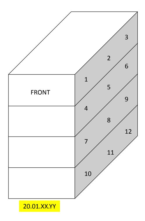
A typical rack in the -20. The numbers on the side is the box number location. Under the rack is a yellow label indicating the address.
