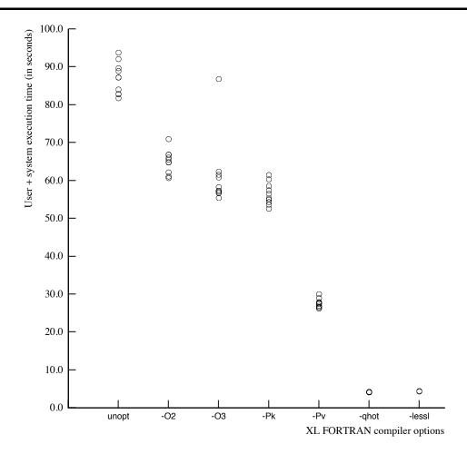
Performance measurements on a 133MHz PowerPC 604 processor for matrix multiply-transpose example.
