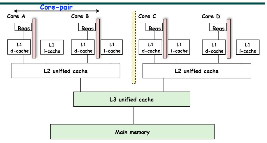
Memory hierarchy for a single Intel Xeon Quad-core E5440 HarperTown processor chip
