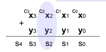
This is the pen and paper addition of two 4-bit binary numbers **x** and **y**. **c** represents the generated carries. **s** represents the produced sum bits.
