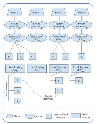
Figure 9: The Distributed Selector System
