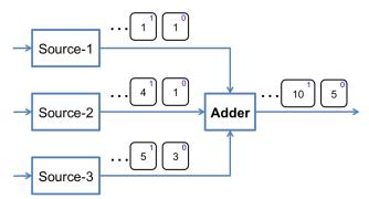
Figure 4: Actor network simulating a join pattern. Source-1, Source-2, and Source-3 are producers for data streams. The Adder actor aggregates data items from each of the three sources and sums them up.
