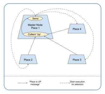
Figure 10: Bootstrap process of a distributed selector program.
