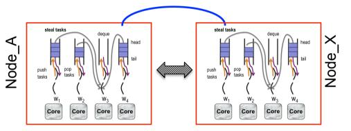
One process with a thread pool at each node
