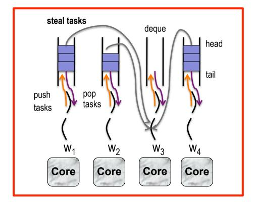
Work-stealing in a thread pool
