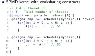
• Race between read of A[i] in S1 (i = 1) and write to A[i] in S2 (i = 1)
