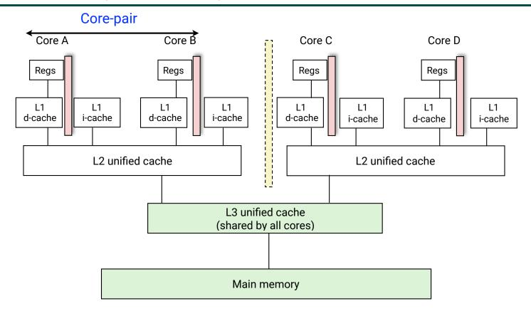
Memory hierarchy for a single Intel Xeon (Nehalem) Quad-core processor chip
