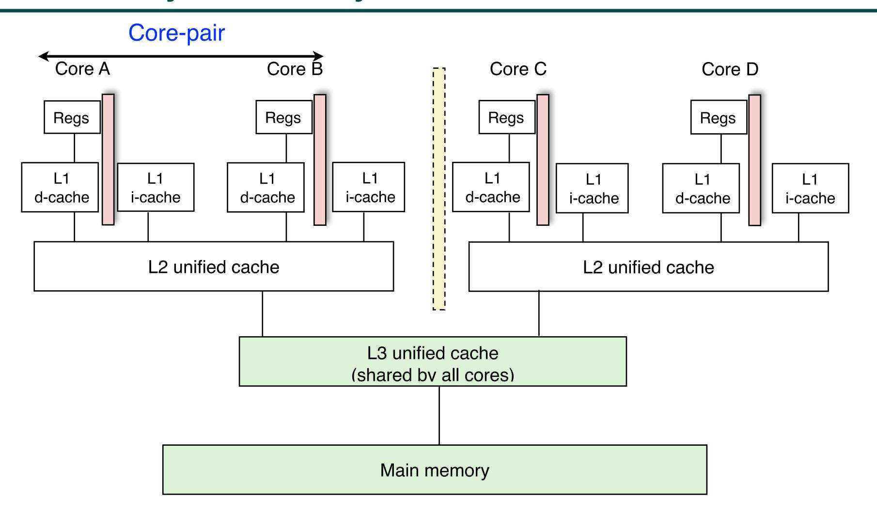
Memory hierarchy for a single Intel Xeon (Nehalem) Quad-core processor chip
