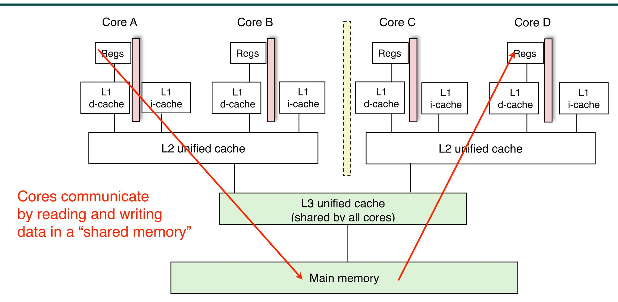
Memory hierarchy for a single Intel Xeon (Nehalem) Quad-core processor chip - A NOTS node contains TWO 8-core or 12-core E5-2650 v2 lvy Bridge chips, for a total of 16 or 24 cores
