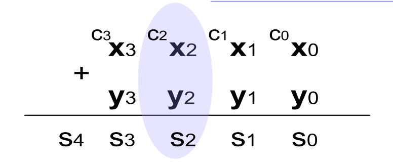
This is the pen and paper addition of two 4-bit binary numbers **x** and **y**. **c** represents the generated carries. **s** represents the produced sum bits.
