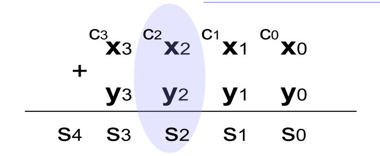
This is the pen and paper addition of two 4-bit binary numbers **x** and **y**. **c** represents the generated carries. **s** represents the produced sum bits.
