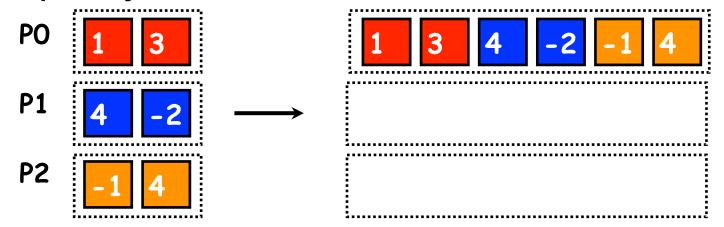
Note: only process 0 (P0) needs to supply storage for the output
