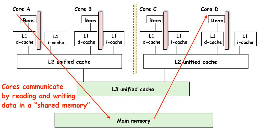
Memory hierarchy for a single Intel Xeon (Nehalem) Quad-core processor chip
