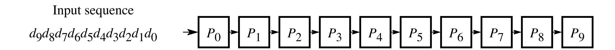
Assuming that the inputs d<sub>0</sub>, d<sub>1</sub>, . . . arrive sequentially, pipeline parallelism can be exploited by enabling task (stage) P<sub>i</sub> to work on item d<sub>k-i</sub> when task (stage) P<sub>0</sub> is working on item d<sub>k</sub>.
