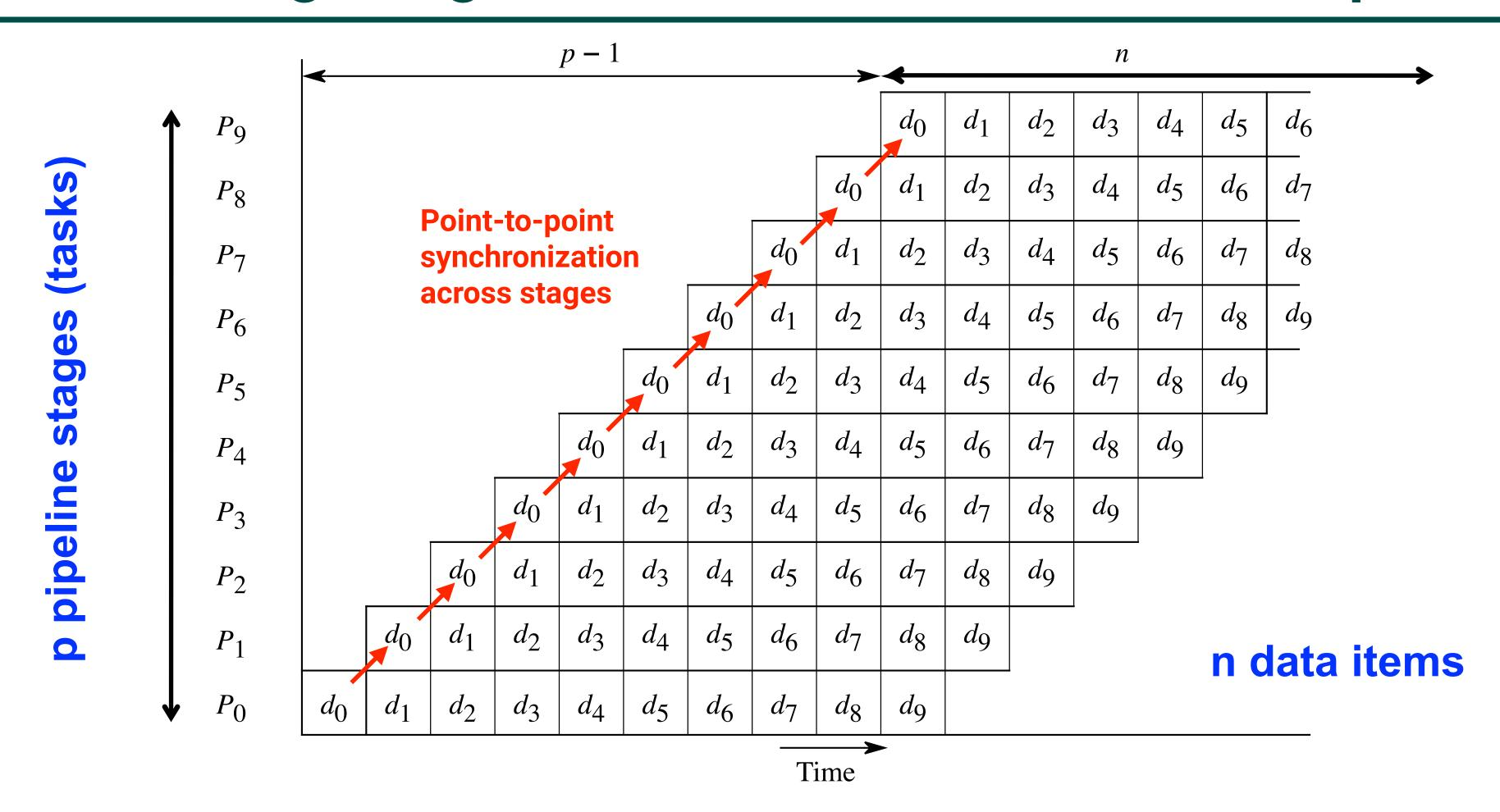
Horizontal axis shows progress of time from left to right, and vertical axis shows which data item is being processed by which pipeline stage at a given time.
