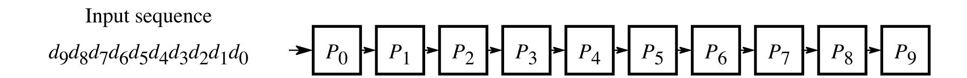
Assuming that the inputs d<sub>0</sub>, d<sub>1</sub>, . . . arrive sequentially, pipeline parallelism can be exploited by enabling task (stage) P<sub>i</sub> to work on item d<sub>k-i</sub> when task (stage)
