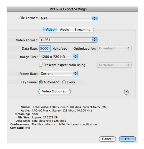
Make sure Video Format is H.264, Data Rate is 5000 kbits/sec, Image Size is 1280x720 HD, Frame Rate is Current, Key Frame is Automatic. If all your settings are the same as the picture shows, click on OK to export.
