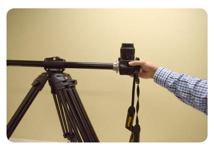
**10.** Screw the camera or video camera directly onto the 1/4" thread.
