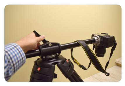
**11.** Turn the lever on the sidearm to loosen the pole
