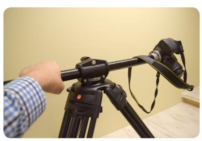
**12.** Turn the pole to the desired angle and then tighten the lever.
