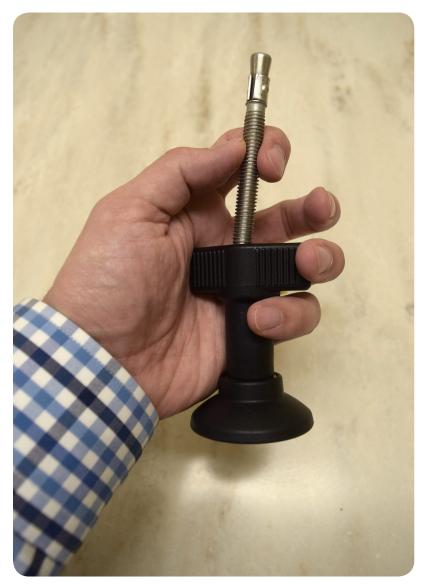
**6.** Insert the 3/8" thread bolt from the side arm package into the tightening handle from the Manfrotto tripod.
