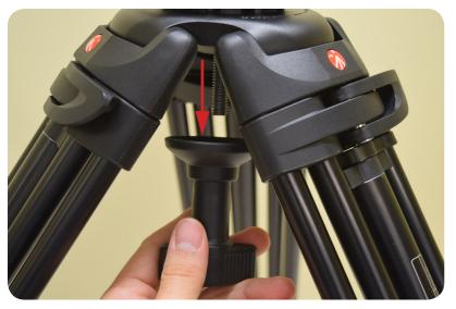
**3.** Unscrew the tightening handle to remove the fluid head. The fluid head will not be used but keep the tightening handle for setup on page 3.
