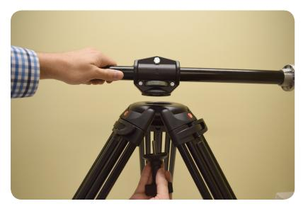
**8.** Set the sidearm onto the tripod and screw in the tightening handle from the bottom.
