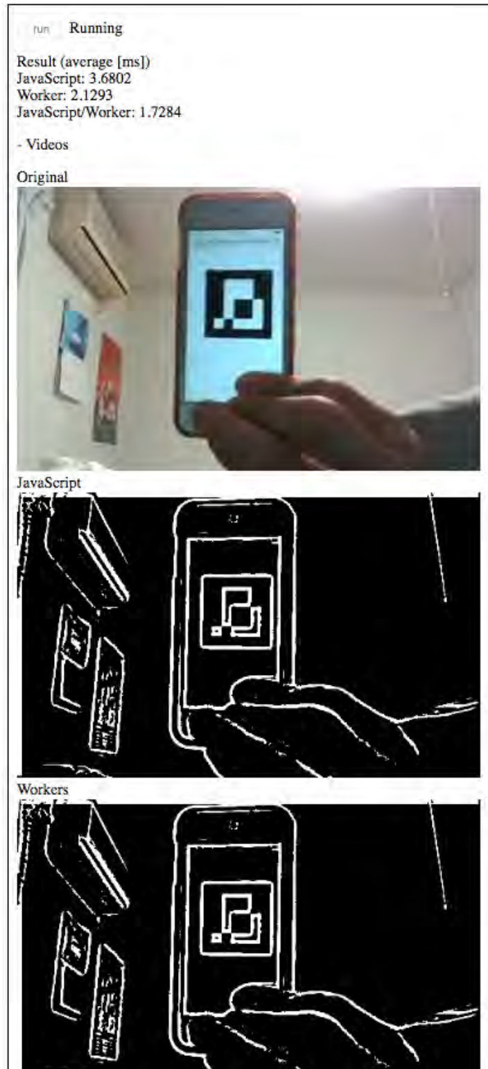
Figure 5.3 : Using Video Threshold detection in threejs using webworker and without using webworker
