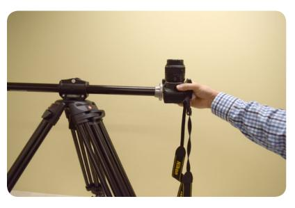
**11.** Screw the camera or video camera directly onto the 1/4" thread.
