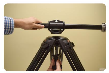
**9.** Set the sidearm onto the tripod and screw in the tightening handle from the bottom.
