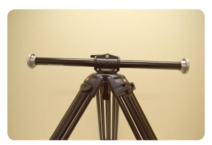
**10.** Turn the sidearm to the desired location before tightening all the way.
