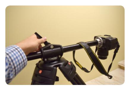
**12.** Turn the lever on the sidearm to loosen the pole
