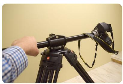
**13.** Turn the pole to the desired angle and then tighten the lever.
