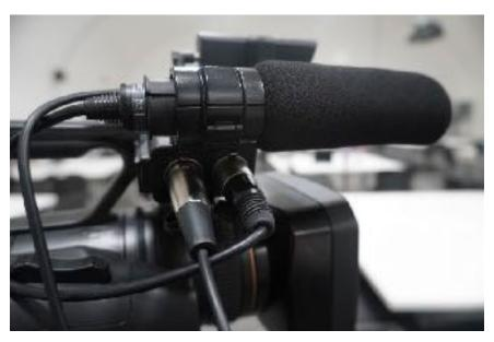
For the microphone side of the XSW-D, set it up on the microphone stand near the presenters and point it at them. Depending on the constraints of the room, you may have to get creative with its positioning. Make sure that the transmitter is plugged into the mic and both it and the receiver on the camera are turned on.
