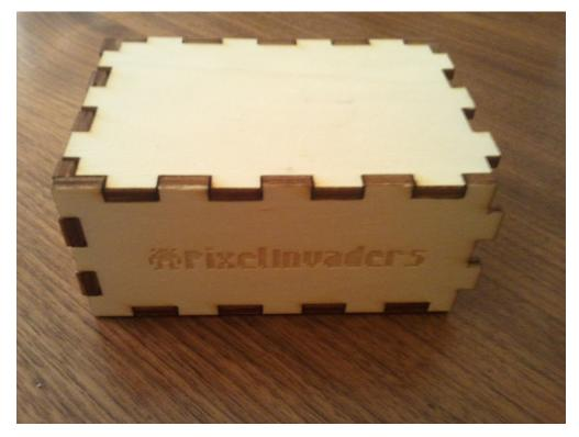
That picture pretty much sums up the finger method. You make little slots and little grooves that connect to each other. The only downside is that you will likely need a little adhesive to keep the sides together since the grooves are not exactly tight.
