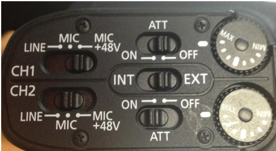
5. Monitor the audio input level on the LCD screen, if everything is connected properly in above steps, you should see audio come from both channels: CH1 should show the level from external shotgun mic, CH2 should show the audio level from wireless microphone. Then use the audio level control to adjust the audio level and make sure the audio meter falls between -20db and -10db.
