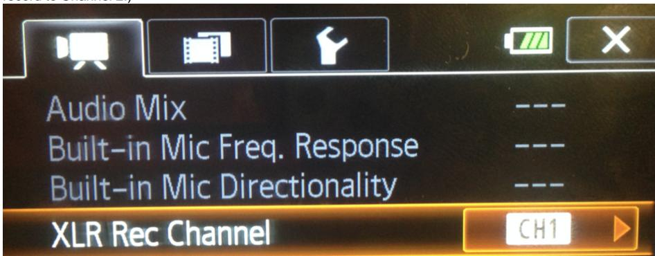
3. Make sure the external shotgun microphone that comes with the checkout package is connected to CH1; then connect any of above recommended microphone to CH2.
